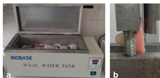
Figure 4: a) Samples stored in a water bath, b) Performing of shear bond strength (SBS) test.
